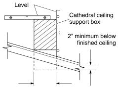
Cut hole 1/8" larger than support box when projected onto roofline
